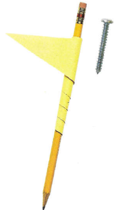
Figure 9 If you could unwind a screw, you would see that it is actually a very long inclined plane.
