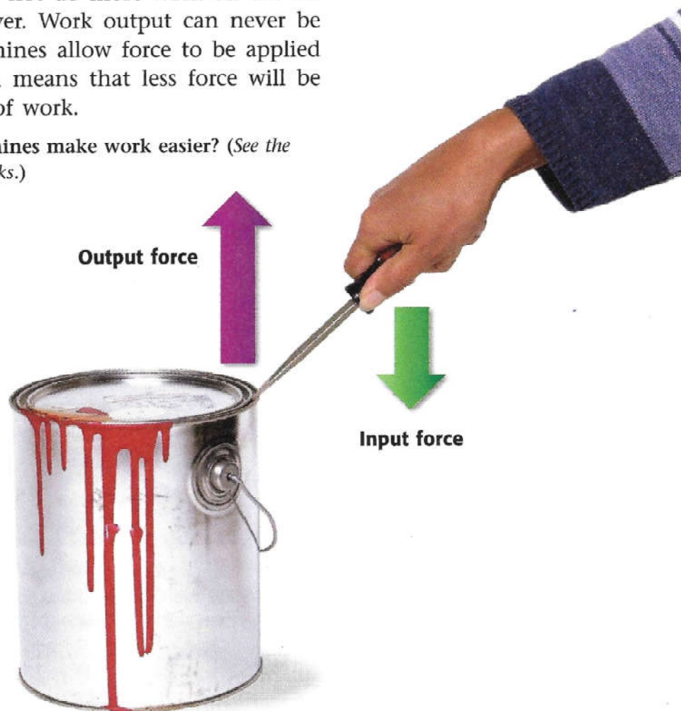
Figure 2 When you use a machine, you do work on the machine, and the machine does work on something else.
